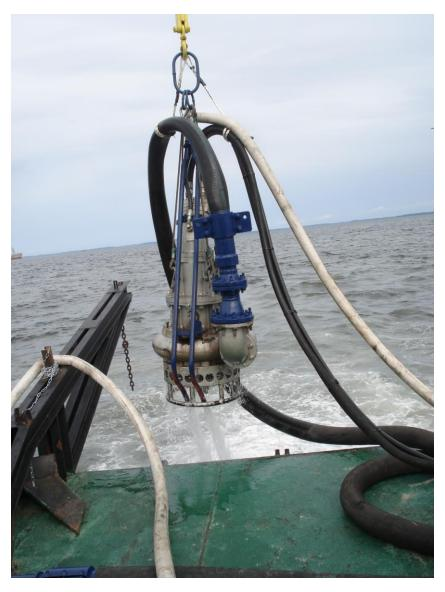
Toyo performance ratings are based on pumping water at specific gravity of 1.0 - if intending pumping slurries then there is need to multiply the horsepower requirement by the S.G of fluid to get the same performance. This is where the hydraulic drive comes in useful because hyd. pressure can be turned up to maintain output flow performance for the heavy slurries.
